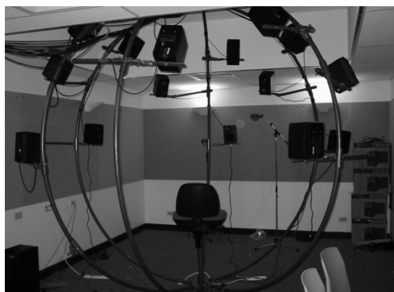
Figure 1. Configurable Hemisphere Environment for Sound Spatialisation (CHESS)
