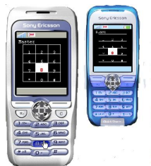
Figure 2 shows a single key ("8") pressed on the master device (larger phone). The corresponding key appears in the MIDlet which displays the pressed key on both the master and the slave devices.
