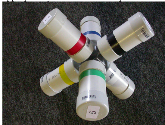
Figure 1. First prototype version of the Didactophone using off-the-shelf plumbing fittings
