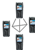
Figure 7. An ad hoc connection system makes connections only when required
