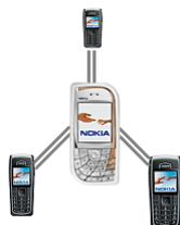
Figure 5. A mobile 'server' configuration allows any player in the ensemble to affect sound on other phones
